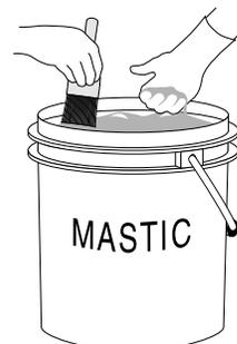
*Tapes do not provide a lasting seal. Mastic is economical, easy to apply and provides a durable seal.*
