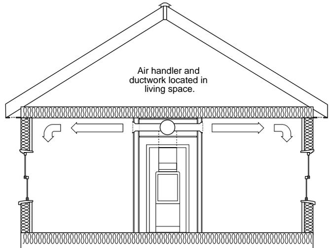
*A Durham, NC affordable housing group locates ductwork in a hallway chase. The chase is sealed with drywall on all sides. The design reduces construction costs and saves energy.*
